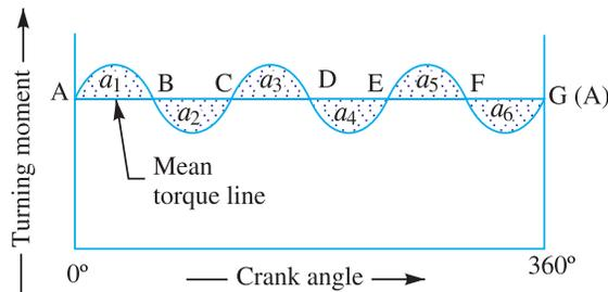
Fig. 22.4. Turning moment diagram for a multi-cylinder engine.
